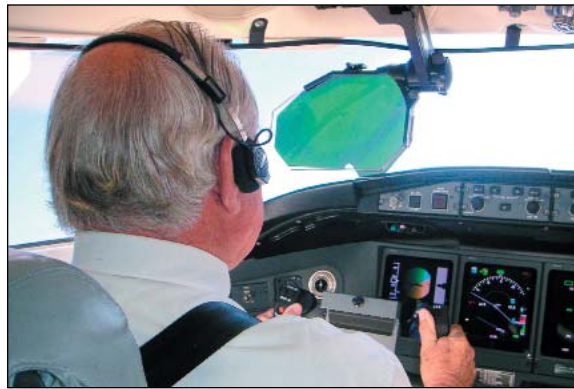
The Thales HFDS was comfortable and intuitive enough for Lacy to fly with it during the entire 1.5-hour flight.
