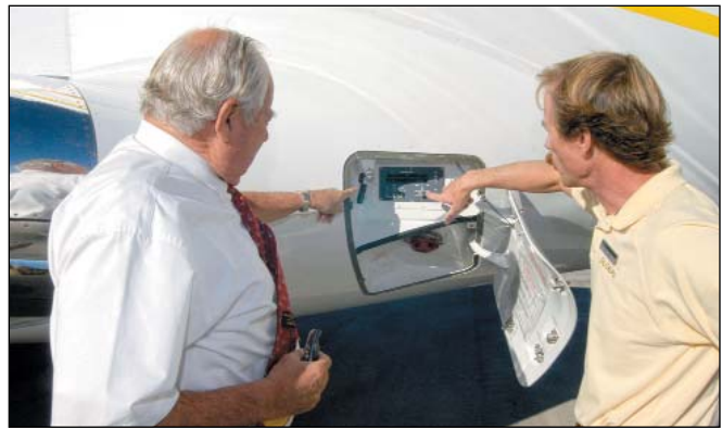
Lacy (L) and Boyd inspect the Global 5000's digital pre-select fuel panel on walkaround at HND prior to departure.
