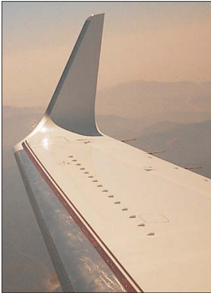
Standing 44 in tall, widesweep blended winglets offer an increased wing area and a reduction in drag.
