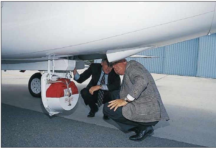
During the walkround Clay Lacy found the 800XP to be very accessible. A ventral access door that leads to the aft fuselage equipment bay (above L) and the easily accessible weather radar (above R) added to the ease of inspection.
