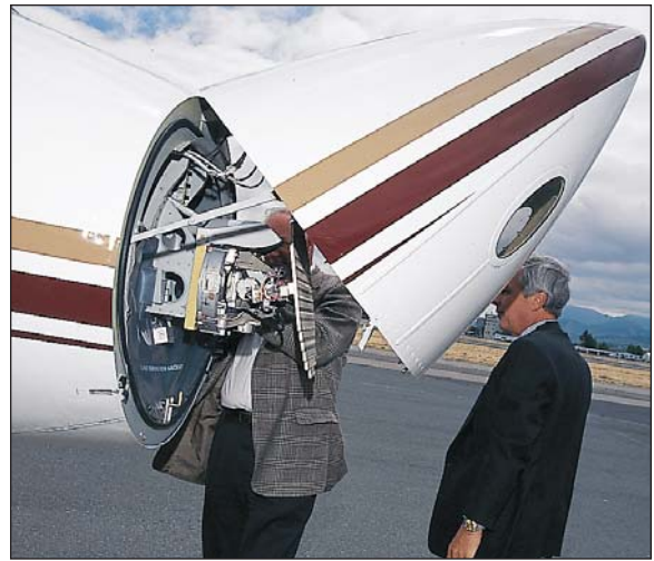
During the walkround Clay Lacy found the 800XP to be very accessible. A ventral access door that leads to the aft fuselage equipment bay (above L) and the easily accessible weather radar (above R) added to the ease of inspection.
