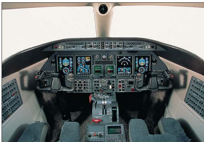
(L) The Learjet 45's Honeywell Primus 1000 integrated panel includes four 8 x 7-in EFIS displays, a Universal UNS1C FMS and a Honeywell Primus 600 weather radar. Aircraft are delivered RVSM capable. Other options include a second Universal FMS, Honeywell EGPWS and TCAS II. (R) A double club passenger configuration is the aircraft's most popular seating arrangement.
