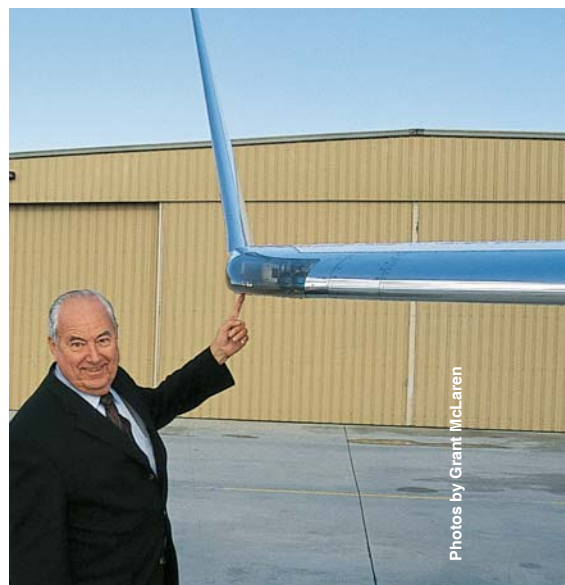
Angular winglets on the GIVSP differ somewhat from the wider-sweep curved winglet design used on the GV.
