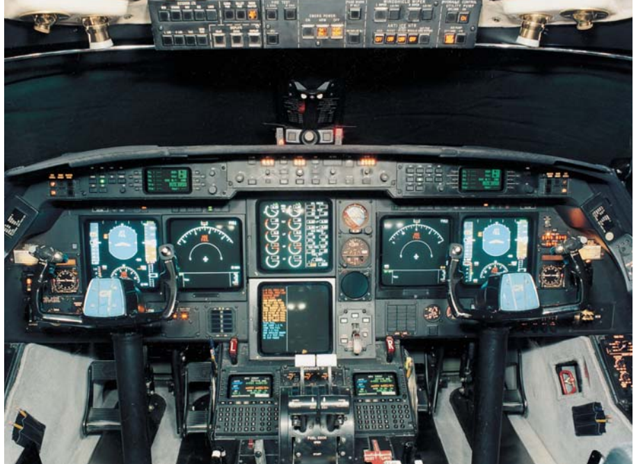
GIVSP features Honeywell's SPZ8400 integrated avionics suite with 6 cathode ray tube displays. Gulfstream plans to offer its new Honeywell Primus Epic-based PlaneView cockpit as an option.
