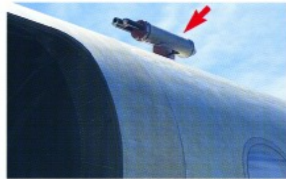
The flight test aircraft, s/n 504 (above), was fitted with a water droplet measuring device used for icing tests.
