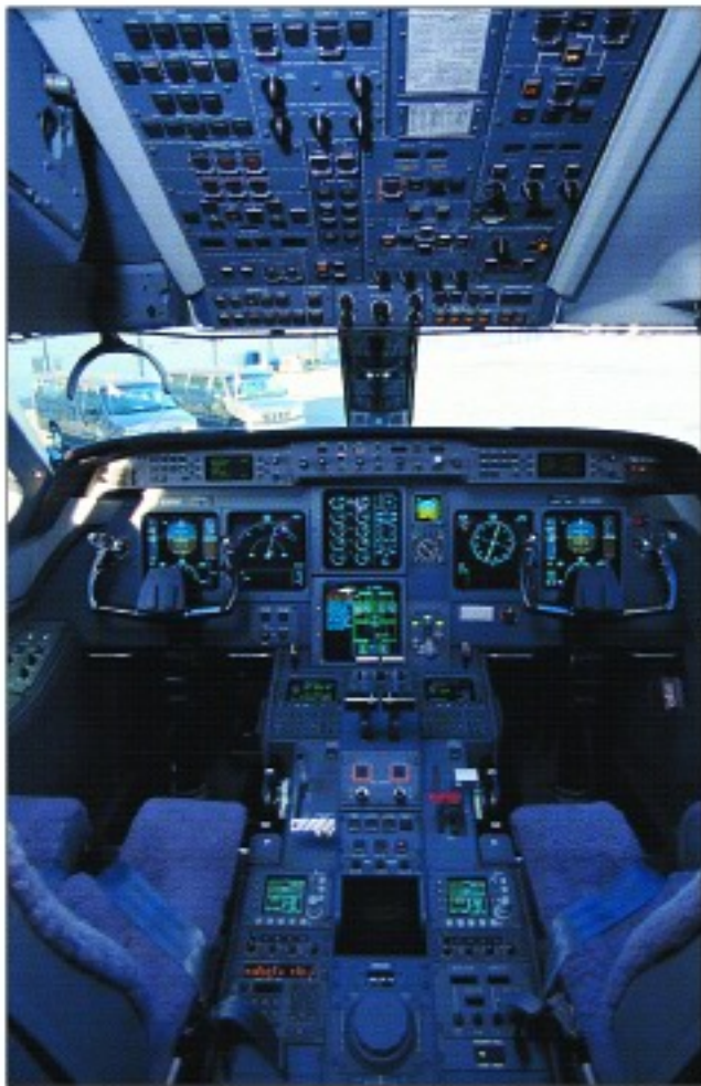
The GV flightdeck features a Honeywell SPZ-8500 panel and a triple-wide pedestal (l). A spacious 16-passenger layout is a typical completion format (upper R). Quiet BMW Rolls-Royce BR710 turbofans provide 14,750 lbs of thrust per side (lower R).
