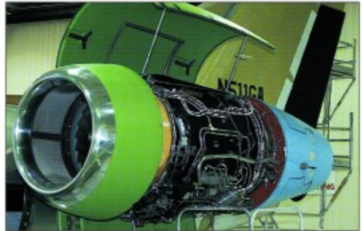
The GV flightdeck features a Honeywell SPZ-8500 panel and a triple-wide pedestal (l). A spacious 16-passenger layout is a typical completion format (upper R). Quiet BMW Rolls-Royce BR710 turbofans provide 14,750 lbs of thrust per side (lower R).
